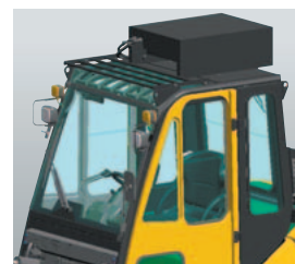
Steel cabin with cooler
