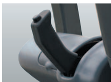
A double action type brake lever to prevent mishandling
