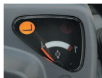
Lifting interlock lamp on the meter panel
