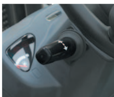
Finger-tip operation with the electric F/R lever
