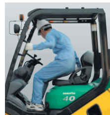
When the operator leaves the seat, Operator Presence Sensing system is activated
