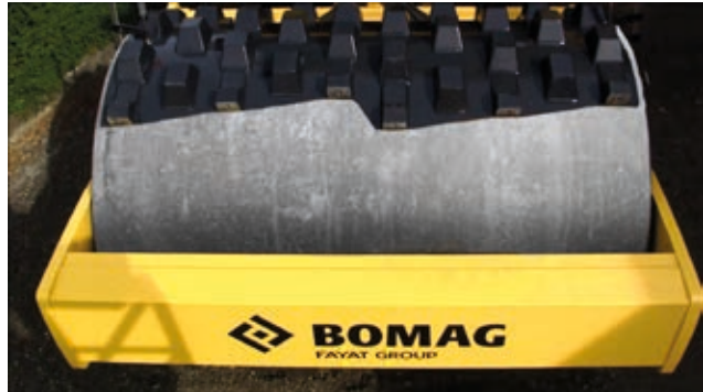
Quick changeover from smooth drum to padfoot drum for flexible working.
