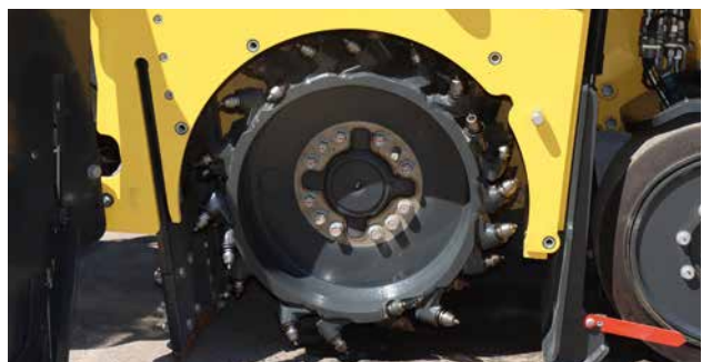
The easily accessible service switch opens the milling box and moves the BM/15 series machines into a convenient servicing position.
