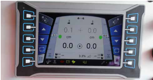
The user interface of the BOMAG Easy Level levelling system display.
