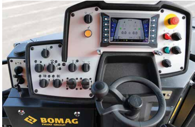
All at a glance: adjustable operating console with 7" full-colour
