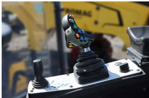
All in the operator's hand: multifunctional travel lever.
