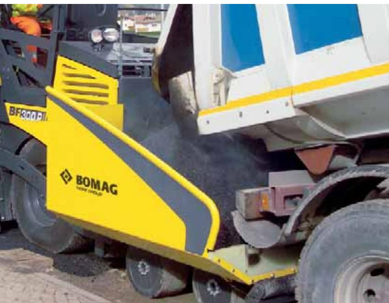
The amply-sized hopper opening makes re-charging from trucks quick and easy.
