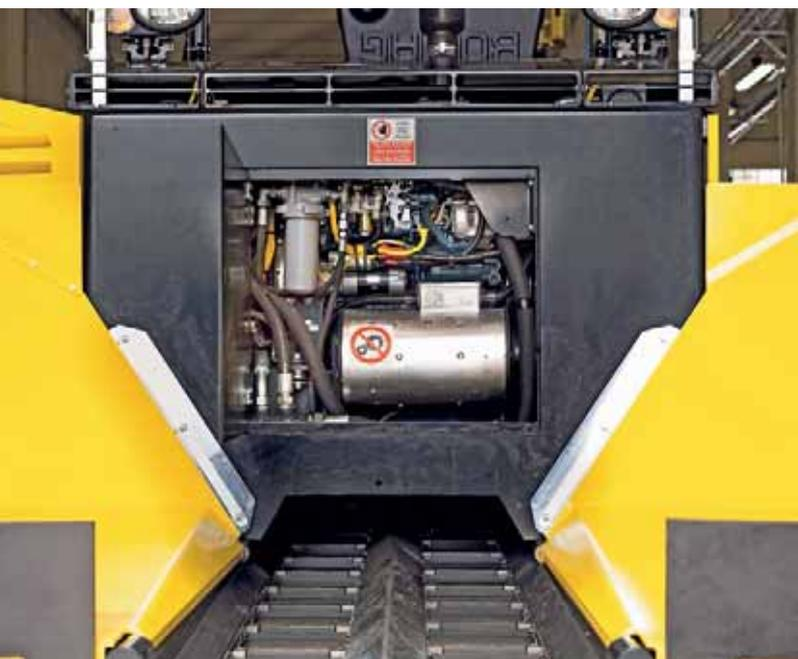
A 3-phase alternator with an output of 13 kW cuts heat-up time.
