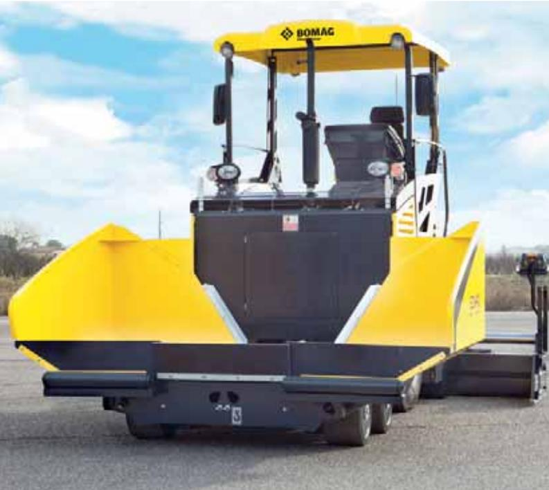
The 9 tonnes hopper capacity means this paver keeps working when others wait to re-charge.
