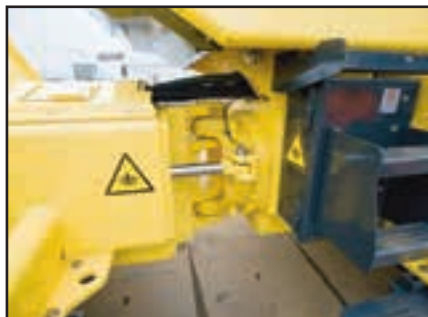
Oscillating center articulation joint ensures ground contact by all four wheels.
