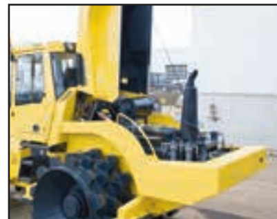
Efficient component access from the vertically opening hood.
