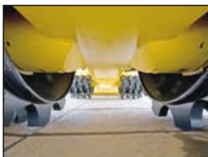
Smooth undercarriage fully protects drive components.
