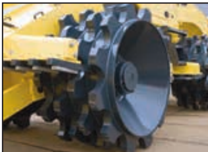
Soil compaction wheels with adjustable scrapers in front of and behind each wheel.
