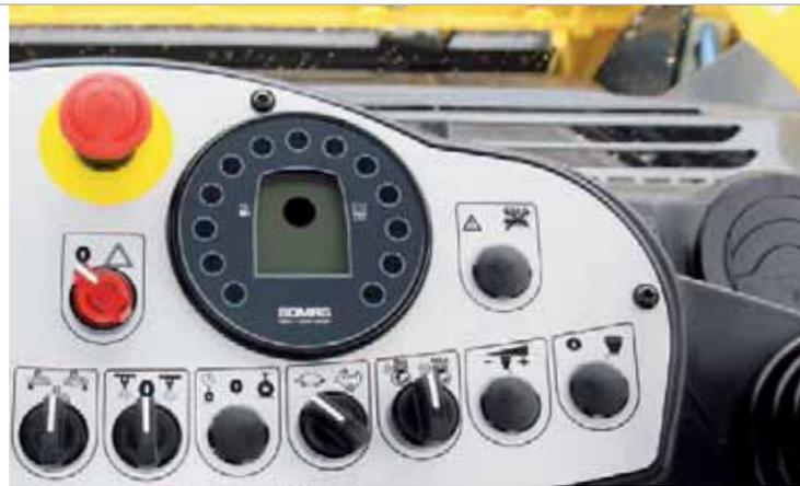
Safety: emergency stop switch and warning lights are arranged centrally.
