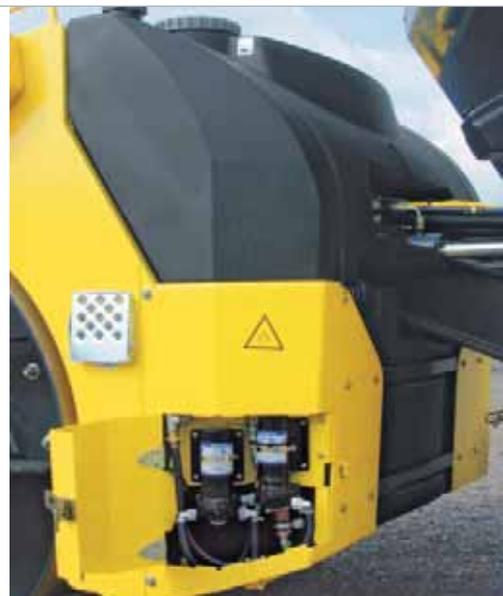
High capacity tanks for less filling stops; two pumps.
