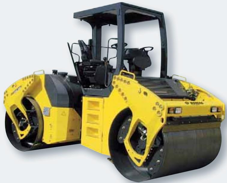
Safety: operator's position with rail and ROPS/FOPS.
