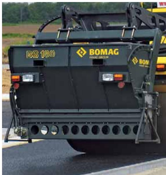
The BS 180 chip spreader for precise and even spread.
