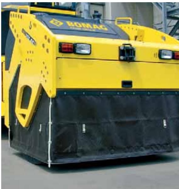
Thermal apron: keeps tyres on combination rollers warm for longer.
