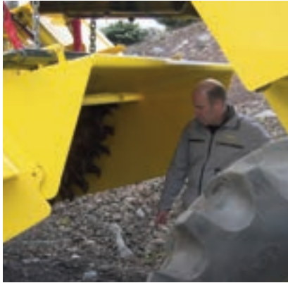
Excellent accessibility for rotor maintenance
